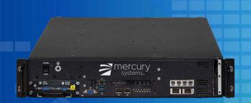
A part of the *EnterpriseSeries*, Mercury's fanless RES Aero 2U Server employs Intel® Xeon® E5-2600 processors to silently accelerate compute intensive workloads for airborne applications such as surveillance, signal intelligence, sensor fusion, and audio/video processing.
