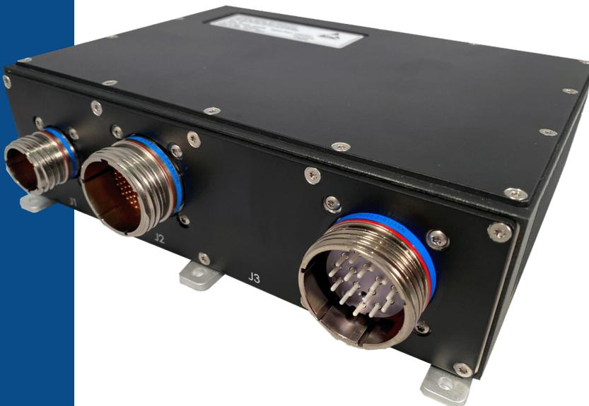
**MC-VCM: Flyable Multichannel Video Converter Module for ARINC 818**
