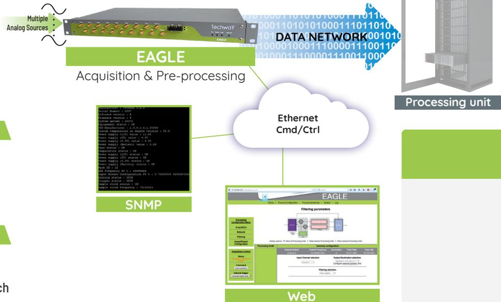
EAGLE is a unique solution which allows to manage multi-channels acquisition and to offload data pre-processing stages from real-time calculators. EAGLE shares the processed data with the communication network making this acquisition solution highly-scalable.
