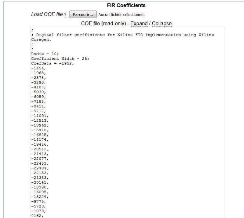
Figure 5: FIR filter's coefficient set loading through WEB interface
